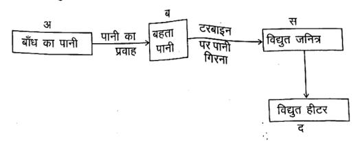
Following flow chart shows the energy production by water. See the flow chart and identify the transformation of energy in (a), (b), (c), & (d).
